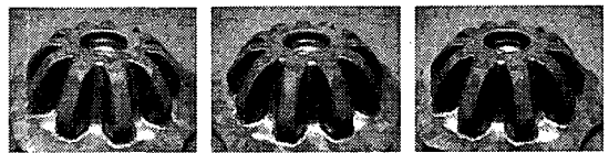
Fig. 3(a) Warm forged bevel gear according to each surface roughness(from left, shot-blasted, turned, polished) with oil-based lubricant (Soy+Graphite)
