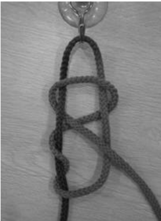
Fig. 3. Hold the end of the loop strand and insert it, under to over, through the space of the two strands, and slightly pull the loop strand.
