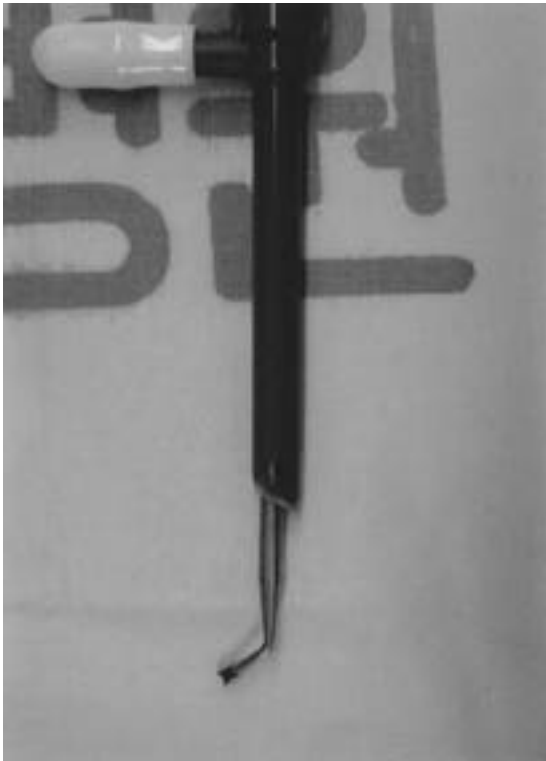
Fig. 3. The anchor is Broken during insertion at lowest hole
