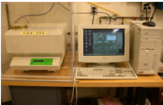
Fig. 9 Thermal Conductivity Testing Apparatus
