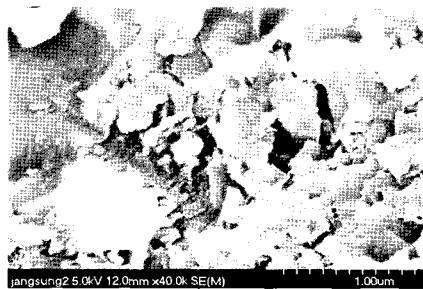
(b) Weathered limestone
