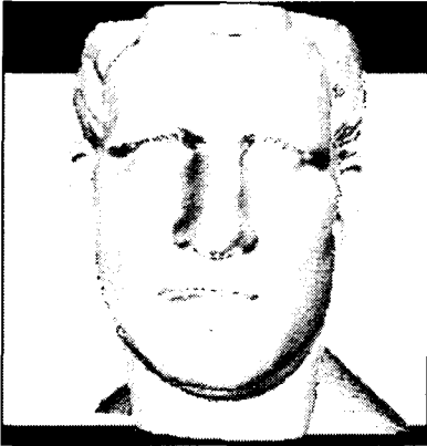
Fig. 10 Measurement result of Agrippa statue by projection moiré
