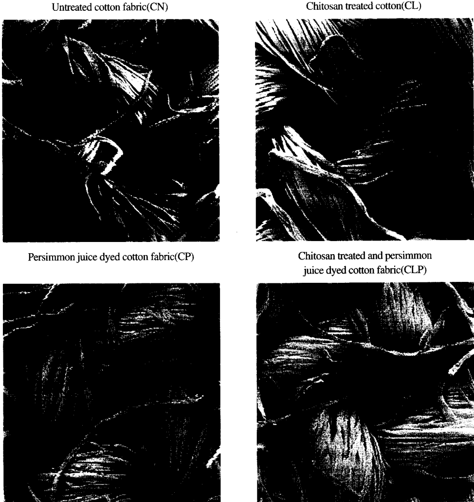
<Fig. 1> The scanning electron micrographies of the untreated, the chitosan treated, the persimmon juice dyed and the chitosan pretreated persimmon juice dyed cotton fabrics (Mag = 50×)
