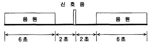
Fig. 3. Configuration of sound sources
