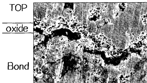
Fig. 2. SEM micrograph of specimen after 24hours holding at 1000℃
