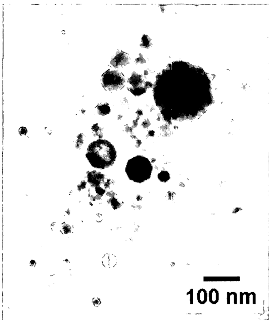
Fig. 1. TEM micrograph of \gamma -Fe 2 O 3 nanopowder used for magnetic core of magnetic photocatalyst.
