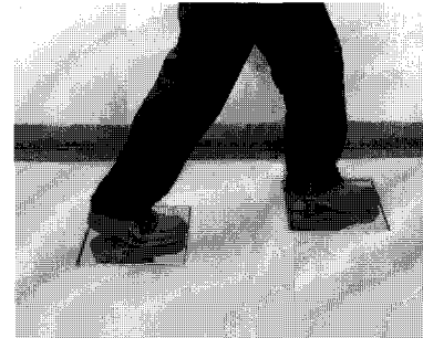
<Fig. 3> Measuring of dynamic load due to pedestrian walking
