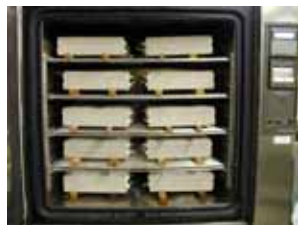
Figure 4. Corrosion Accelerated Curing [ Chamber ].
