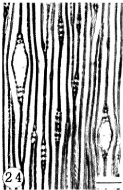
Fig. 24~26. Fusiform rays in tangential surface. -24: Compression wood. -25: Lateral wood. -26: Opposite wood. Scale bars = 100 \mu m.
