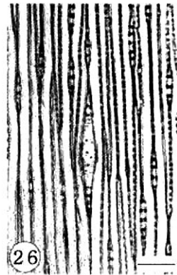
Fig. 24~26. Fusiform rays in tangential surface. -24: Compression wood. -25: Lateral wood. -26: Opposite wood. Scale bars = 100 \mu m.
