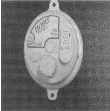
Figure 2. HOBO, Measuring instrument for temperature and relative humidity
