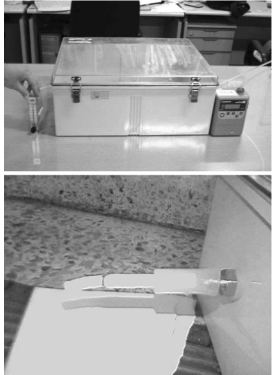
Fig. 1. The collection of ETS sampling using the lung vacuum sampler.
