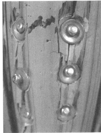
Fig. 6. Wood block shear failure.
