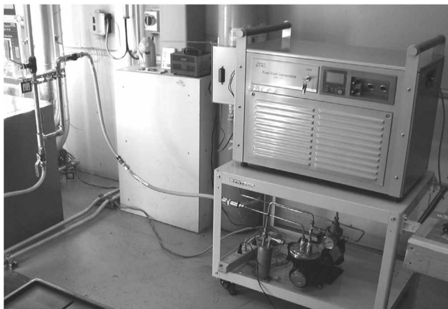
Figure 13. Biogas PEMFC Generator connected to the biogas model plant in Obihiro University.
