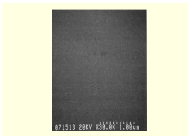
Fig. 1. SEM image of \text{AlO}_x thin film deposited at 80°C using 500 cycles.
