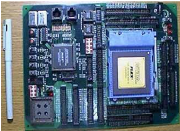
Fig. 8. FPGA test-board for tests on number of iterations ( E_b/N_0=1 dB).
