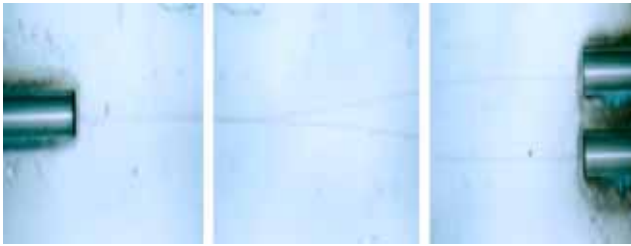
Fig. 4. Fiber-aligned one-input and two-output channels of U-grooved optical splitter.
