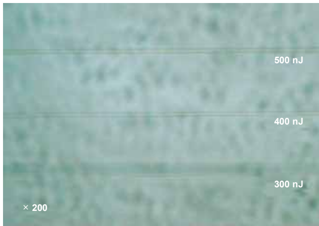
Fig. 1. Optical micrograph of waveguides written inside fused silica glass using a 300 to 500 nJ, 1 kHz, and 100 fs pulse train focused with a 0.42 NA microscope objective.
