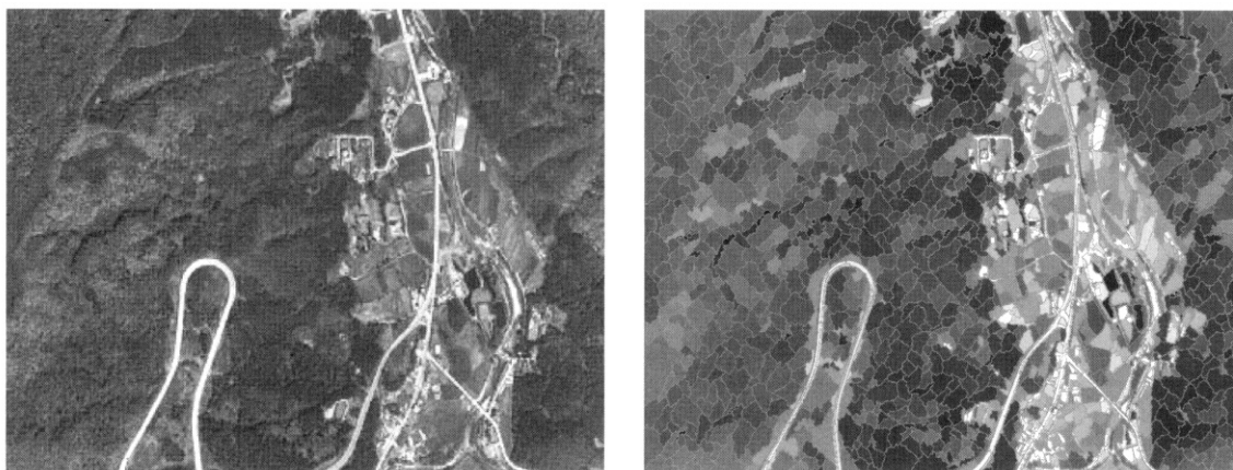
Figure 7. Segmented imagery using digital aerial photograph.
