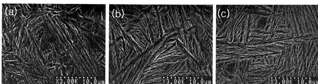
Fig. 5. SEM microstructures of alloys austempered for 21 min at 350°C: (a) 1.8, (b) 2.3 and (c) 3.0 Si.
