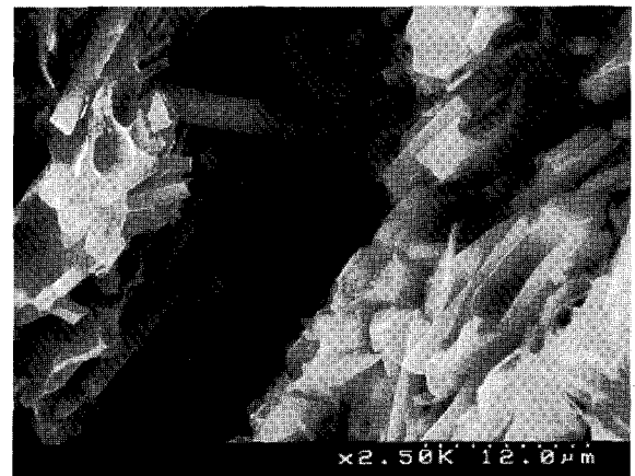
Fig. 8. SEM fractography of Kaowool reinforced composite.
