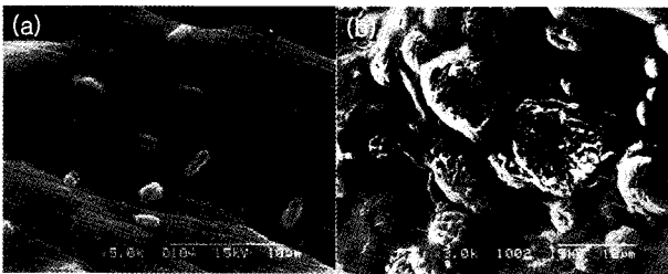
Figure 4. Scanning electron microscopy of immobilized Enterobacter cloacae YJ-1 ((a) Internal surface before fermentation. (b) Internal surface after fermentation).
