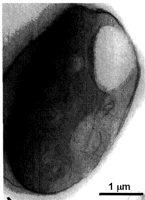
Figure 4. TEM image of a cross-section of a polystyrene fiber electrospun from the 30 wt% DMF solution (16.0 kV/21 cm).
