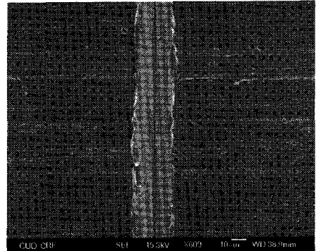
(b) V-grooved surface by OC
