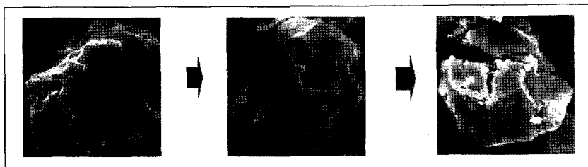
Fig. 3. Oxidizing behaviour of non-irradiated UO_2
