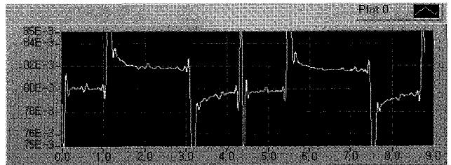
Fig. 13. The signal distortion due to electromagnetic induction inside the multi-interphone cable in the resistivity survey.
