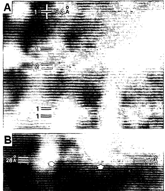
Fig. 5. (A) 1-2 talc layers are interlayered within chlorite layers. (B) Transformations of two chlorite layers (28 Å) into two talc layers (18.6 Å) are shown within packets of chlorite layers. Transition areas are marked by arrows.
