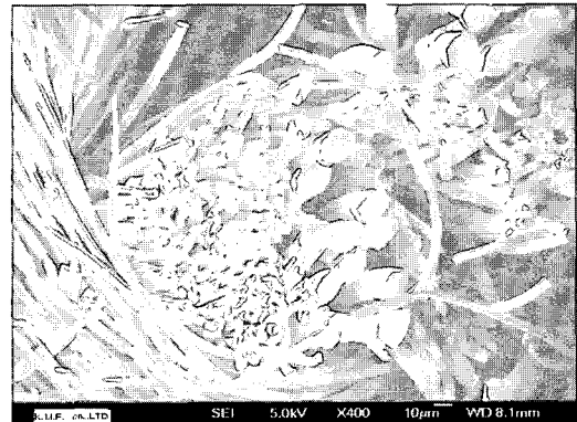
(b) DSPM2 : PET 70d/300f + High shrinkage PET 30d/12f
