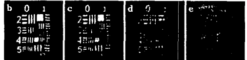
Fig. 8 (a) Measured bit error rates of the images restored for different ratios of wrong cells in the mask: (b) 0%, (c) 15%, (d) 30%, (e) 50%.
