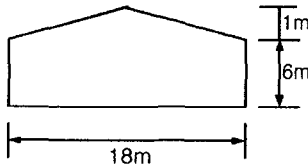
(c) Front view of tunnel with gable roof
