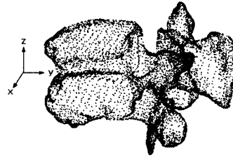
Fig. 8 Point data orientation of the spine optimized for SLS using the proposed algorithm
