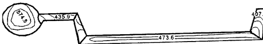
Fig. 4 Part temperature field after at the end of solidification (6 seconds of cooling) considering diffusion heat transfer at interface part/mould
