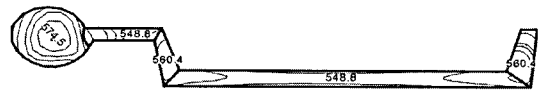
Fig. 6 Part temperature field at the end of solidification (14,8 seconds of cooling) considering Newtonian heat transfer at interface part/mould
