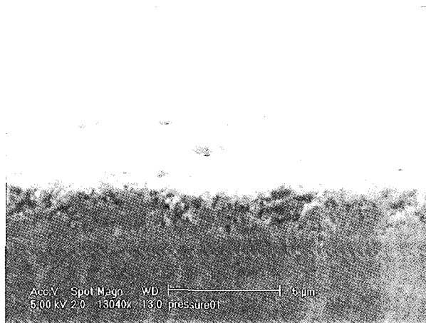
Fig. 3. The SEM images of pore morphology and overall porosity. A; Top and side view after 3 min etching time B; Top and side view after 10 min etching time.
