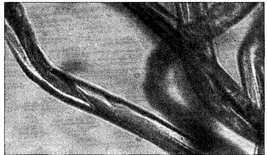
Fig. 13. Optical microscope photograph( \times 200 ) of acetate fiber used as tobacco filter.
