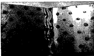
Fig. 18(b) Failure shape of ISB panel with the woven metal (Upper surface)
