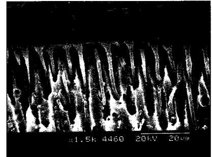
Figure 8. SEM photograph of the adhesive interface of CFS group ( \times 1500 ).
