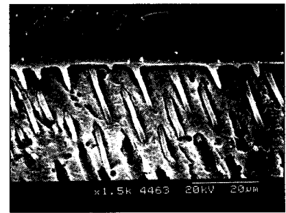
Figure 14. SEM photograph of the adhesive interface of DFS group ( \times 1500 ).
