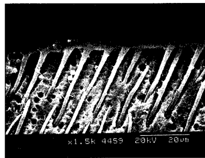
Figure 13. SEM photograph of the adhesive interface of DFO group ( \times 1500 ).
