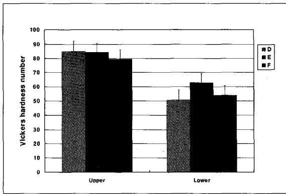
Fig. 6. Mean microhardness values(Vicker's hardness, Number) of group D, E and F group at upper and lower surface
