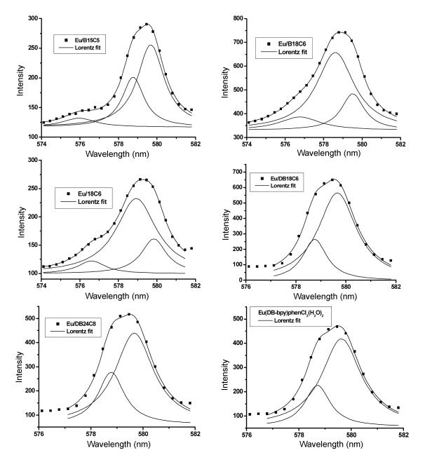
Figure 5. Lorentzian fitting curves of  ${}^{5}D_{0}$ - ${}^{7}F_{0}$  emission bands for Eu(DB-bpy)phenCl<sub>3</sub>(H<sub>2</sub>O)<sub>2</sub> and the composite systems with crown ethers.
