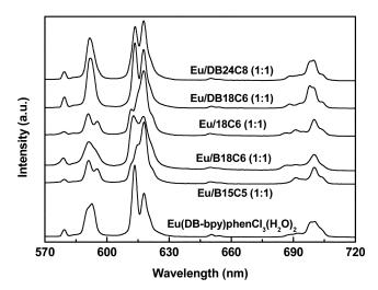
Figure 4. Typical emission spectra of  $Eu(DB-bpy)phenCl_3(H_2O)_2$  and the composite systems with crown ethers.
