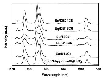
Figure 2. Typical emission spectra of  $Eu(DN-bpy)phenCl_3(H_2O)_2$  and the composite systems with crown ethers.
