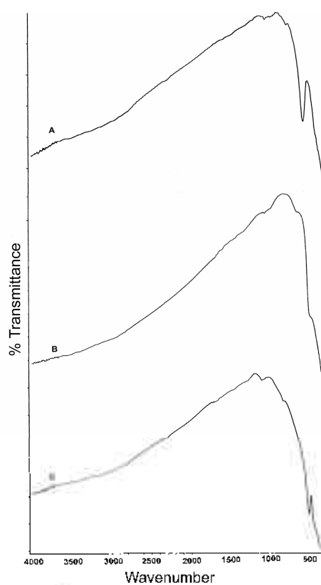
Fig. 5. The final decomposition products of: (A): [La(hip)_3] \cdot 4H_2O , (B): [Ce(hip)_3] \cdot 7H_2O (C): [Sm(hip)_3] \cdot 8H_2O .
