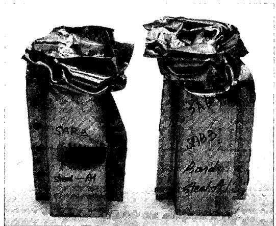
Photo. 2 Deformed shape after the crush test
