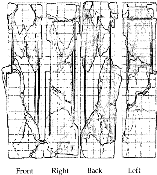
Fig. 13. Fracture formations due to vertical load of 1.0ton(RC2-10-2).
