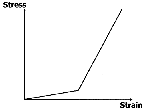
Fig. 2. Predicted stress-strain behavior of rubber connecting system.
