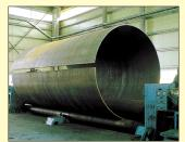
• Roll Bending Pipe(EFW)
