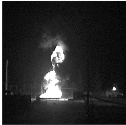
Fig. 11. A picture of pool fire in 25000L storage tank
