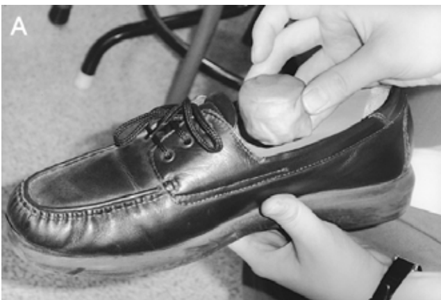
Figure 2. Photographs showing the methods to measure the height of the toe box. (A) Toe box height was measured by placing putti inside the shoe and a mold was made.(B) Mold was removed and measured.
