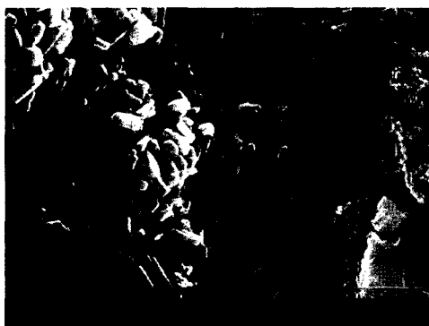
Fig. 9 SEM of SPF-a after 4-week sulfuric acid attack
