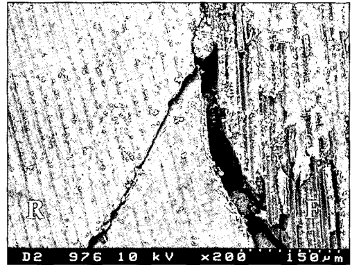
Fig. 8. The interface of glass fiber post and resin core in type D fracture(×200) (F : Glass fiber post, R : Resin core)
