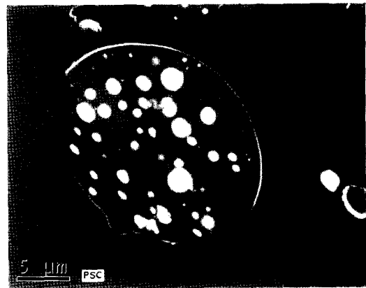
Figure 3. TEM image of TPP microcapsule (B-2) with the multi-core structure containing 33 wt% of TPP contents based on the TPP + epoxy resin.
